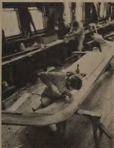
Cutting the rabbet in the keel assembly; the carver's mallet is resting on the centerboard case. Sandy Johnson/Apprenticeshop.
